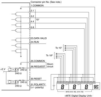
Note: The BCD output connector pin number is the D-sub connector pin number when the BCD Output Cable (sold separately) is connected. This number differs from the pin number for the Digital Indicator narrow pitch connector (manufactured by Honda Tsushin Kogyo Co., Ltd.).
